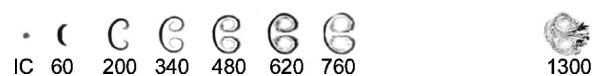
FIG. 1. Composite laser-sheet visualization of the shock-accelerated gas cylinder evolution. Direction of the flow is from left to right. “IC” denotes initial conditions, timings of subsequent dynamic exposures (microseconds after initial acceleration) are labeled.
